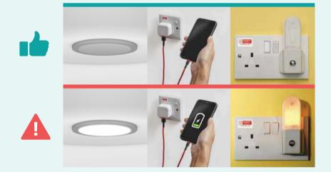
Test all light switches and power sockets in every room. The RCCB is working if your lights and appliances do not turn on.
