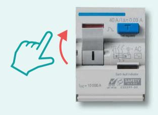
Switch off all lights and power sockets. Flip up the RCCB switch to restore power supply and switch on lights and appliances that you need.
