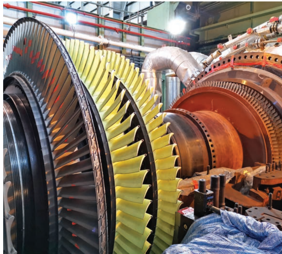
^ One of the gas turbines which Senoko Energy has upgraded with new cooling technologies and advanced materials, such as thickened thermal barrier coating on the turbine blades.
